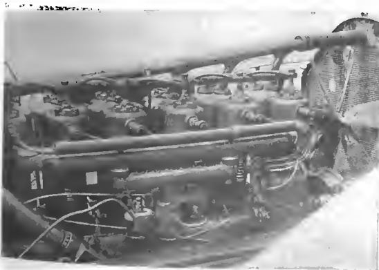
Inlet Side of Motor Showing Manifold Design.
